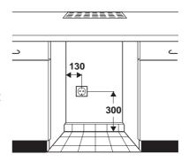
If the socket is not accessible once the appliance is built in, the electrical installation must include suitable means of isolating the appliance from the mains (e.g. fuse, cut-out, current trip or similar with a minimum contact separation of 3 mm).
